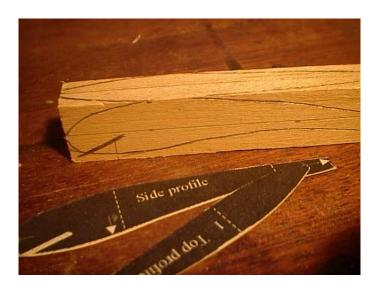
3. Transfer the templates timber blank and rough the lure to shape. You can get more information on how to do this in Make Your Own Fishing Lures
