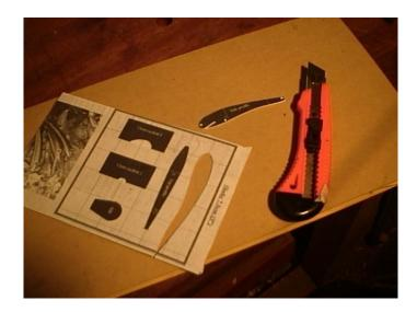
2. Glue the sheet onto the card and use the knife to cut out the templates.
